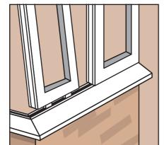
Sill Support Blocks on the panels locate into the sill, and click into position.
