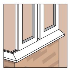
Panels engage into Sill and slide into position.
